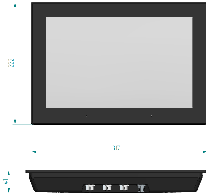
Figure 12: CCpilot V1200 dimensions
